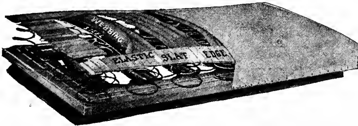
Fig. 3935. SECTIONAL VIEWS, SHOWING THE USE OF SLAT AND WEBBING AND THE ELASTIC SLAT EDGE.
